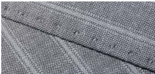
Edging stitch imitating a manual stitch ("AMF seam")
