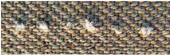
Material damage due to needle penetration
