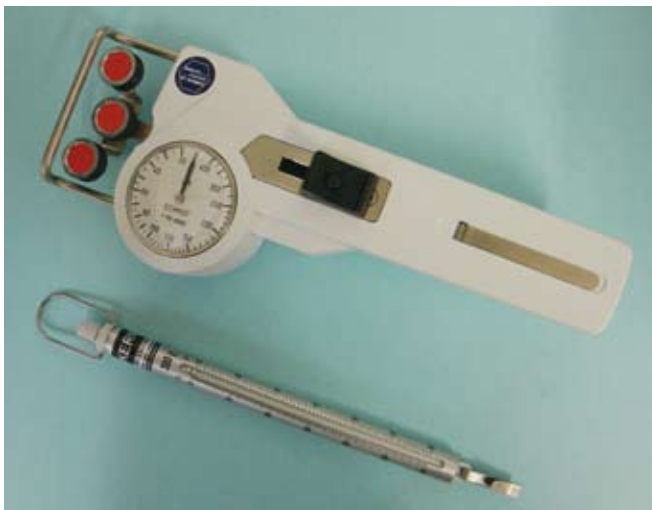
Thread tension meter and spring balance to check thread tension on the sewing machine
