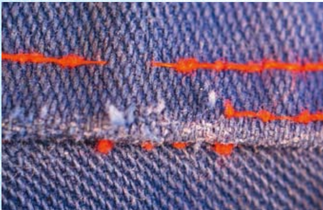
Chafed seams - often reason for complaints with protective or work clothes
