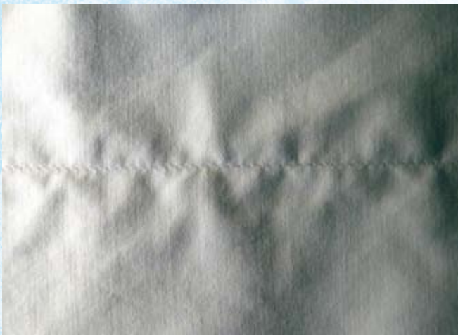
Unacceptable seam look due to too high thread tension
