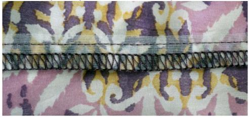
Bonding of the seam line with an inlay
