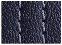
Twin needle seam with S- and Z-twisted thread
