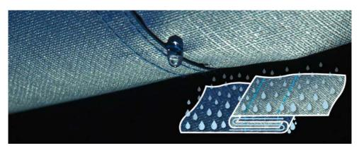
Water leakage with felled seam
