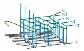
NT = needle thread LT = looper thread CT = cover thread
