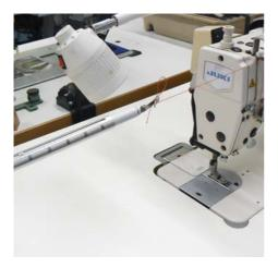
Now, at the position of the take-up lever, the tension measuring device is evenly pulled in horizontal direction to the left (away from the take-up lever).
