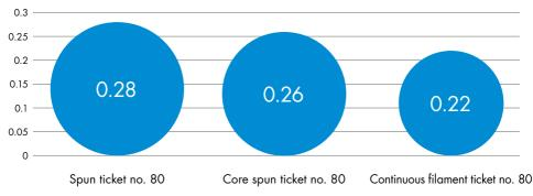
Comparison of the optical diameter with different construction types
