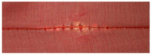
Poor seam strength as a result of slippage
