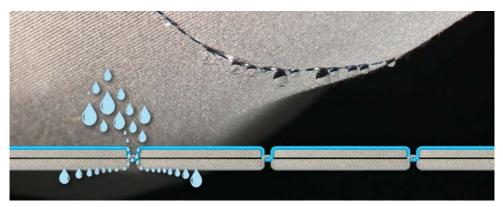
Water leakage with topstitch seam and conventional sewing thread
