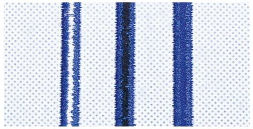
Correct thread tension while embroidering (Bobbin thread is 1/3 of the surface)
