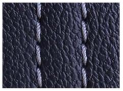
Twin needle seam with 2 Z-twisted threads
