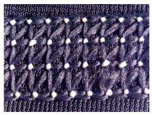
Correct thread balance with stitch type 607: view of the bottom of the seam
