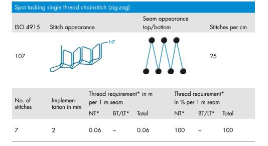
NT = needle thread | BT = bobbin thread LT = looper thread | CT = cover thread
