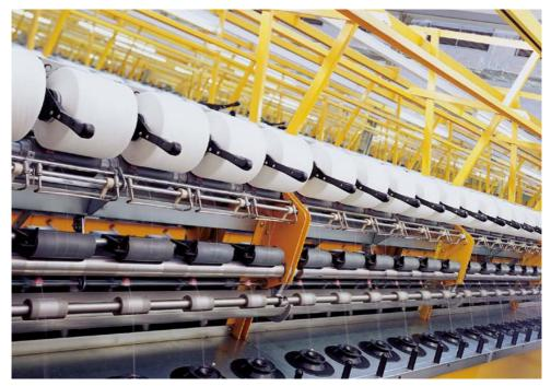
Final twisting machine of a double level twisting unit
