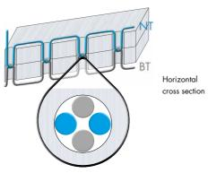
Cross section of stitch interlocking with lockstitch
