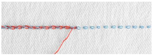
Thread balance after unpicking the seam – needle thread tension is too loose
