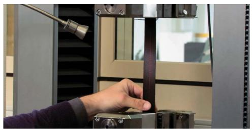
Examination of the seam elasticity with the tension-testing device
