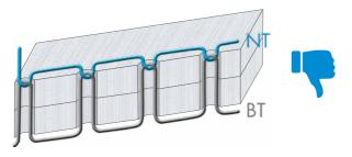
Needle thread tension (NT) too tight or Bobbin thread tension (BT) too loose
