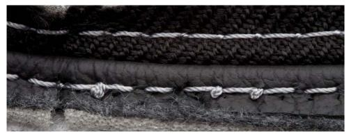
Knots on the lower side of the seam
