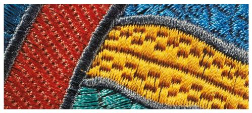
**Fill stitches** fill surfaces. Depending on the stitch rhythm and frequency, the surface can have an increased or decreased glance and show relief-like structures. Selecting the correct stitch length can help to reduce the number of stitches required, thus reducing production time.
