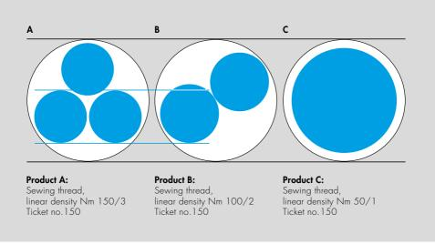
All three products consist of yarns with different linear densities, however, because of the different thickness of the single hanks they have the same final linear density, and therefore carry the same ticket numbers.
