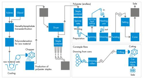
Production of polyester fibres according to the melt spinning process
