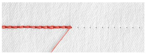
Thread balance after unpicking the seam – needle thread tension is too tight
