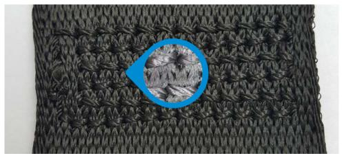
Twisting with multidirectional seam (microscope)
