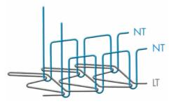
Sketch of stitch type 406 (NT = needle thread, LT = looper thread)
