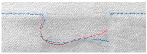
Thread balance after unpicking the seam – both threads are equally long
