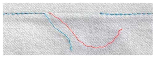
Thread balance after unpicking the seam – bobbin thread is too short
