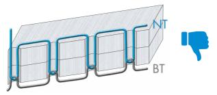
Needle thread tension (NT) too loose or Bobbin thread tension (BT) too tight
