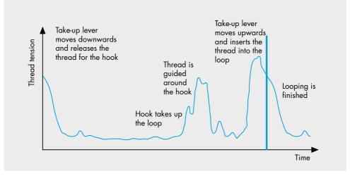
Thread tension during sewing operations
