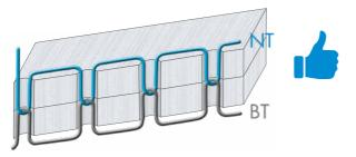
Looping of needle thread and bobbin thread (NT or BT) in the centre of the material
