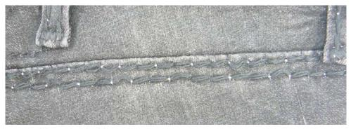
Seams with poor thread balance
