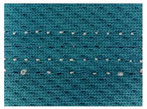
Unfavourable thread balance with stitch type 607: view of the bottom of the seam
