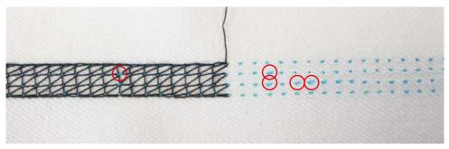
Overturning needle thread loops on the bottom side of the seam with stitch type 607
