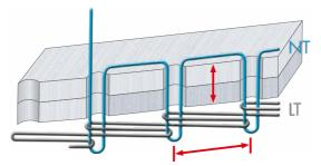
1 stitch = 4× length of the stitch + 2× thickness of the material + thread quantity for interlooping\*
