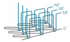
Sketch of stitch type 407 (NT = needle thread, LT = looper thread)
