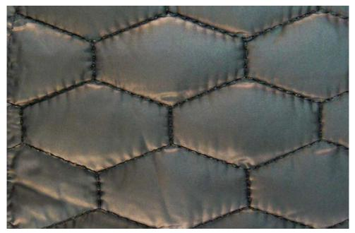
Down jacket sewn with continuous filament, Serafil fine 180 (120/2)
