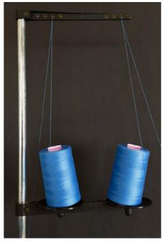
Crocked cones (without spool holder) impair the off-winding performance
