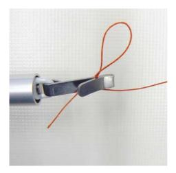
The thread needs to be slightly struck off over the thread guiding in the take-up lever and needs to be fixed in the thread clamp of the tension measuring device.
