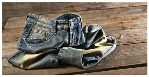
Special wash treatment on jeans (partial sanding, brushing and spraying)
