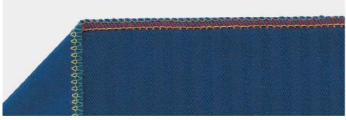
Poor thread balance with stitch type 504
