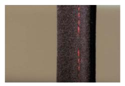
Test object with torn seam
