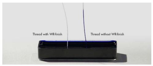
Comparison of capillary effect with thread with WR-finish and normal thread
