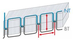
1 stitch =  $2 \times 1$  length of the stitch +  $2 \times 1$  thickness of the material + thread quantity for interlooping\*
