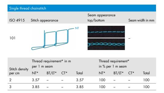
NT = needle thread | BT = bobbin thread LT = looper thread | CT = cover thread
