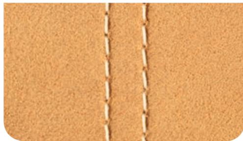
No water stains/dry seam when using sewing threads with WR-finish
